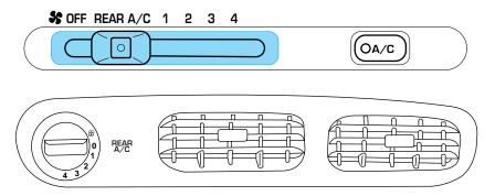
turn the Rear Fan Control on the main climate control system to Rear A/C and turn the Rear A/C Fan Control to 0.
